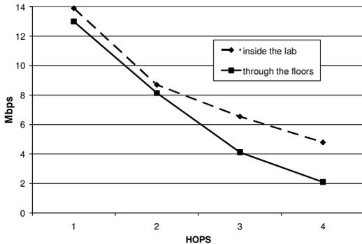
**Figure 15 - Comparison (inside the lab vs. five floors) for UDP**
