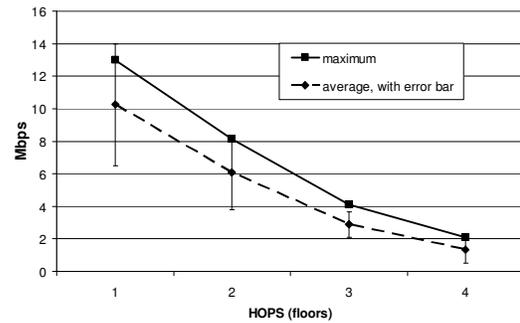
**Figure 14 - Throughput given hops (floors) for UDP**
