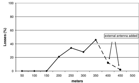
**Figure 9 – Packet Loss given distance for scenario B**
