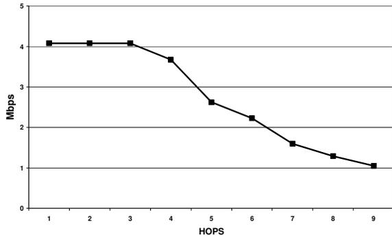
**Figure 12 - Throughput given chain length for SCP**
