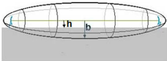
**Figure 5 - Fresnel zone partially obstructed (if  $h$  is smaller than  $b$  there is obstruction)**
