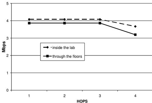
**Figure 16 - Comparison (inside the lab vs. five floors) for SCP**
