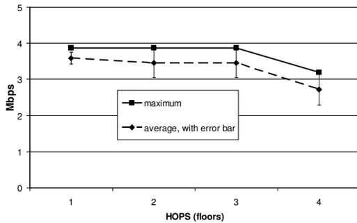
**Figure 13 - Throughput given hops (floors) for SCP**
