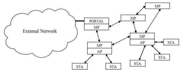
Figure 4 - mesh network architecture
