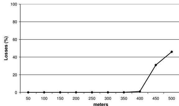
**Figure 7 - Packet loss given distance for scenario A**
