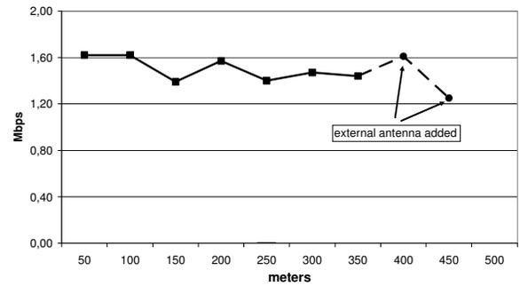
**Figure 8 - Throughput given distance for scenario B**
