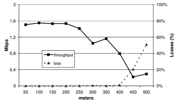
**Figure 6 - Throughput and losses given distance for scenario A**
