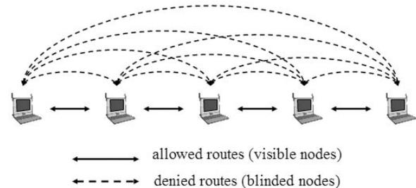
**Figure 10 - A chain of XOs and the Blinding Table**
