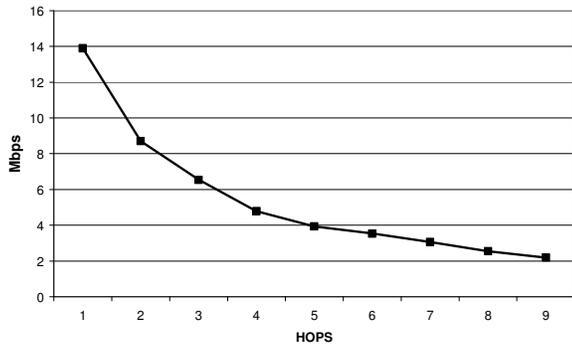
**Figure 11 - Throughput given chain length for UDP**
