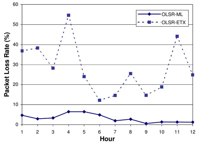
Figure 3: The ReMesh packet loss rate for communications between nodes 3 and 6.
