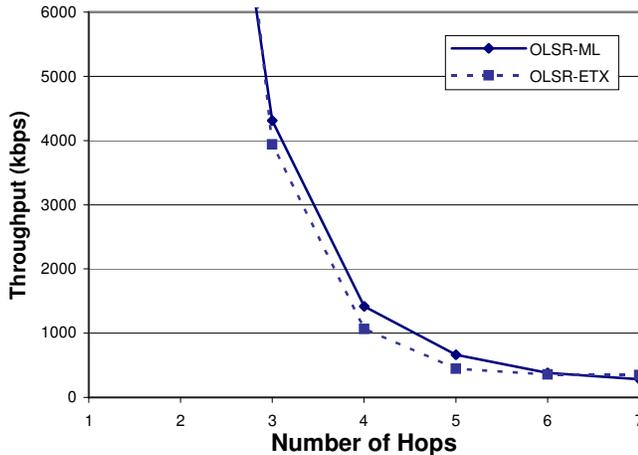
Figure 5: The ReMesh throughput measured with IPERF for communications starting at node 3.
