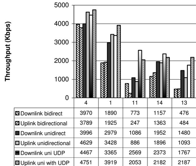
Figure 9: Outdoor throughput measured with IPERF.
