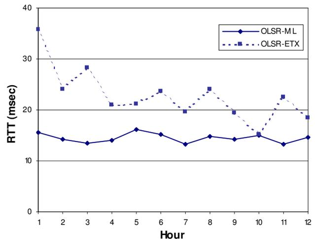
Figure 4: The ReMesh round trip times for communications between nodes 3 and 6.
