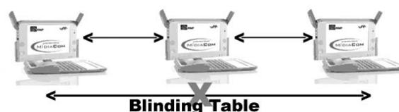
Figure 3 - Blinding table operation – the nodes in the edge must forward their frames through the central node
